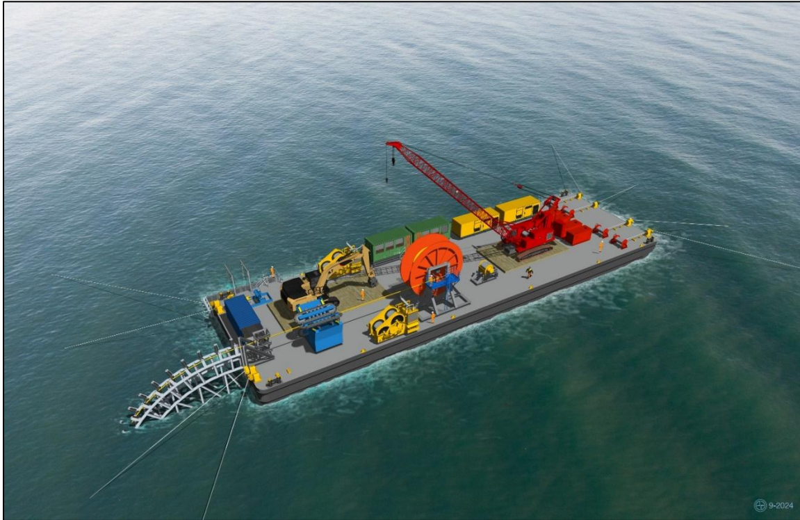
Figure 9. Schematic of Reverse Cable-Lay Barge Support Vessel
