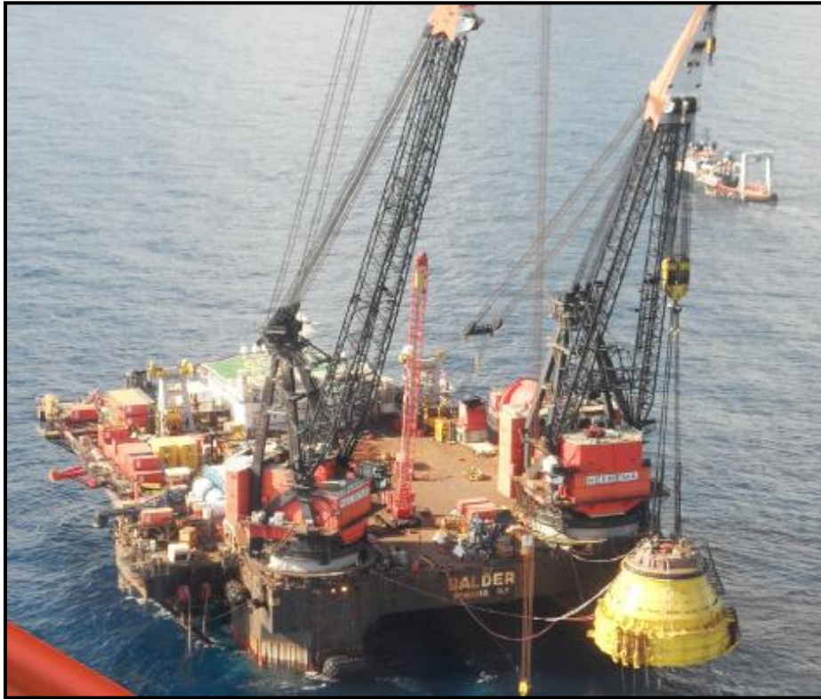
Figure 6. Typical Anchored Heavy Lift Vessel Spread
