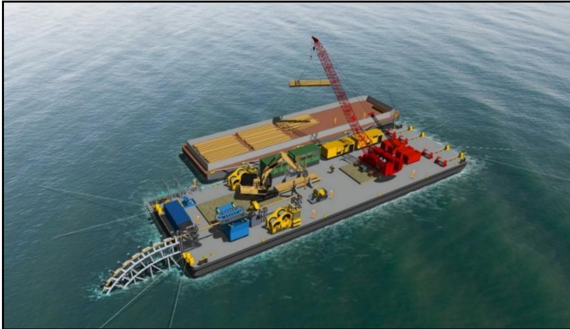
Figure 8. Schematic of Reverse Pipe Lay Barge and Materials Barge Support Vessel
