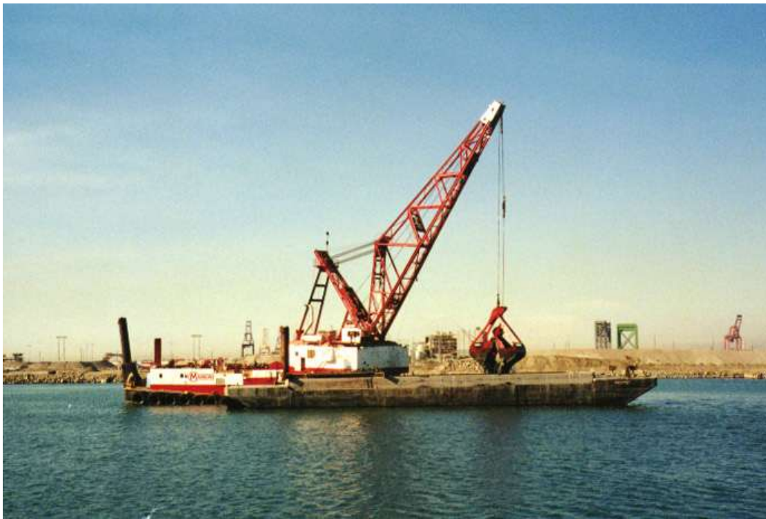
Figure 2-4 Example Photo of a Clamshell Dredge on a Barge
