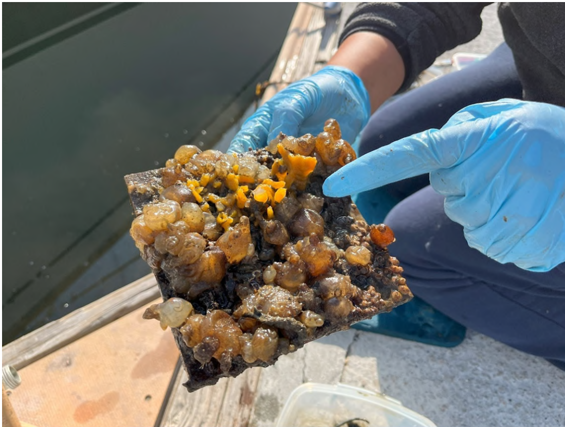
Figure 7-1. Example of plate used by the Smithsonian Environmental Research Center to monitor the presence of organisms in hard surfaces at each location surveyed after 3 months submerged in the water.
