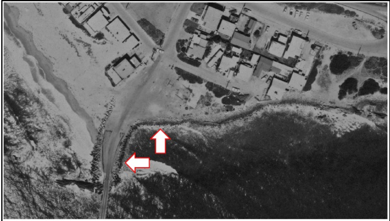
Figure 4.6-4. Riprap Hardscape Present Along SCC Parcel Shoreline (Photo From 1971, Arrows Indicate Riprap Placed Before This Time and Existing Natural Rock )
