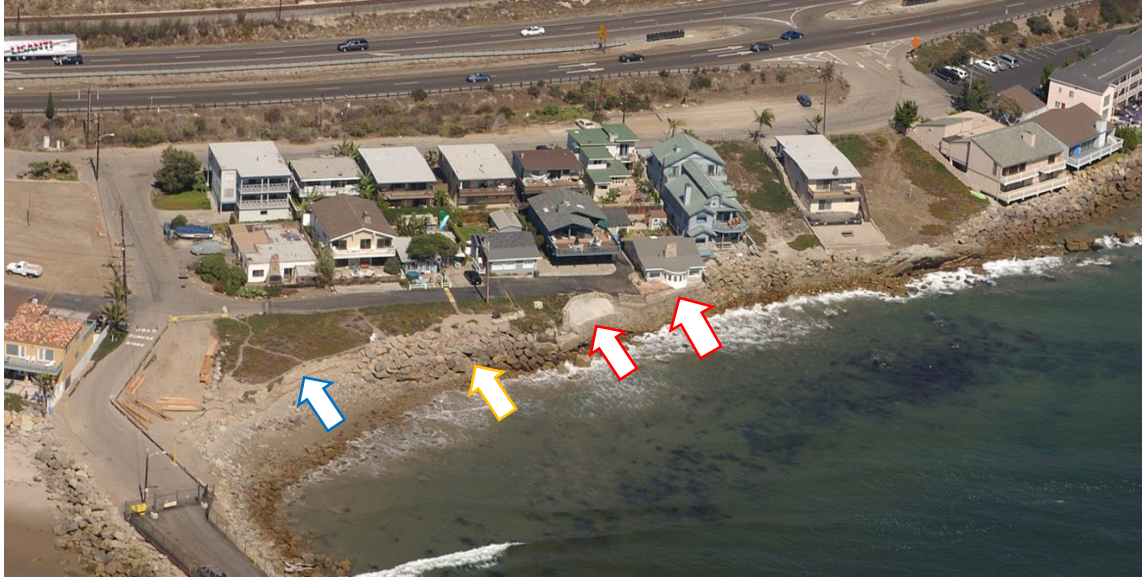
Figure 13. 2002 photograph showing two concrete seawalls at downcoast end of SCC parcel (red arrows) and riprap now added upcoast of the seawalls (orange arrow). The low bluff is now fronted with a scarp along its entire western section (blue arrow) (California Coastal Records Project – Kenneth and Gabrielle Adelman).
