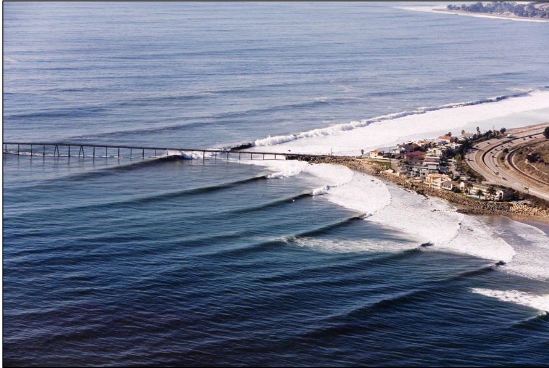
Figure 33. Aerial view of a large swell breaking at Punta Gorda showing no change in waves as they pass through the causeway (© Josh Wolcott).
