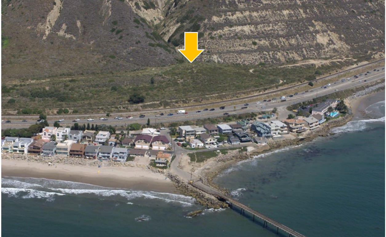
Figure 12. Alluvial fan (at arrow) formed at mouth of arroyo immediately inland from Punta Gorda. (Photo: California Coastal Records Project – Kenneth & Gabrielle Adelman).
