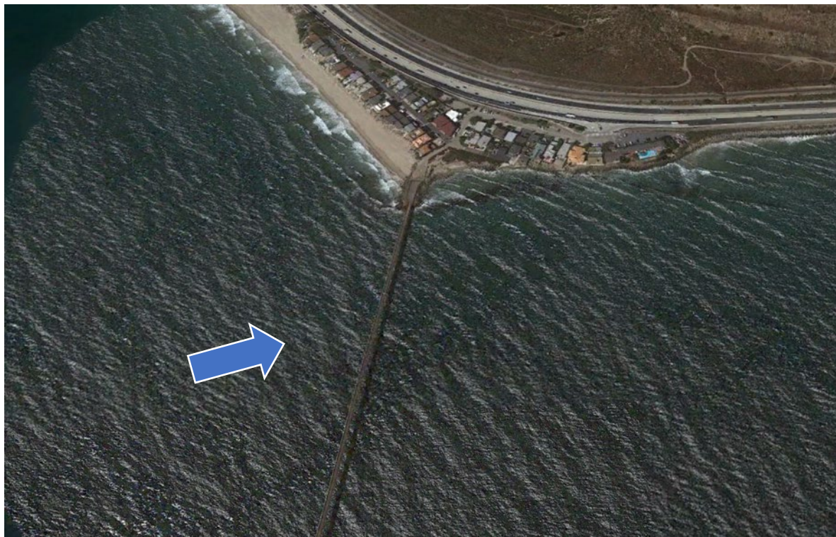
Figure 30. Wave trains from the WSW (from approximately 250°) passing unchanged through the causeway in August 2019.
