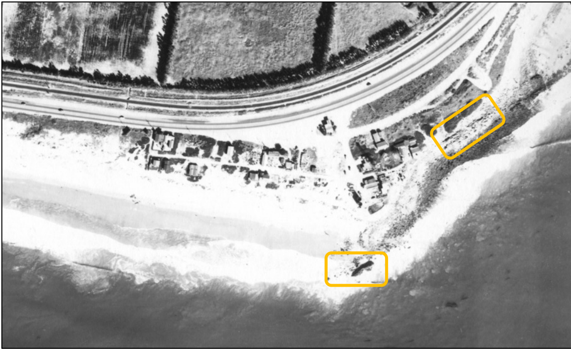
Figure 15. 1944 aerial photograph of Punta Gorda showing Pico Formation outcrop on beach (outlined in yellow) that acts as a groin to trap longshore transport of sand. Additional outcrop occurs on the back beach down coast.
