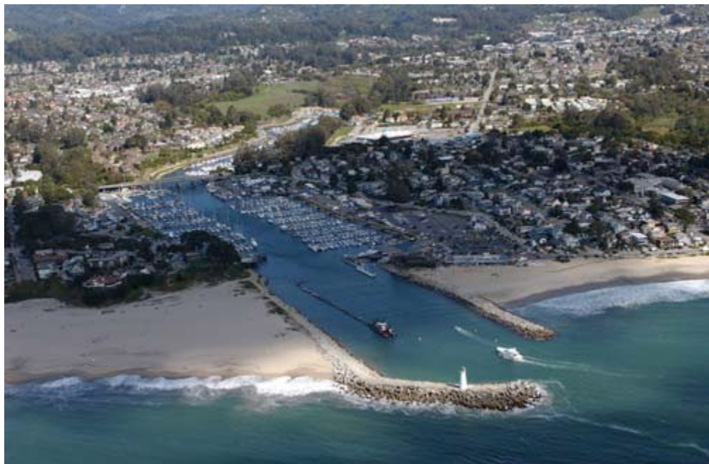
Figure 10: The jetties at the Santa Cruz Harbor interrupt the flow of sediment, creating a wide beach immediately upcoast of the harbor but depleting downcoast beaches. Credit: Copyright (C) 2002-2023, Kenneth & Gabrielle Adelman, California Coastal Records Project, www.Californiacoastline.org
