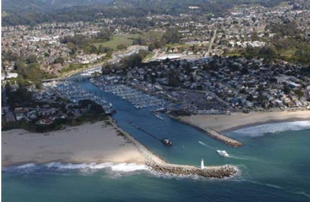
Figure 10: The jetties at the Santa Cruz Harbor interrupt the flow of sediment, creating a wide beach immediately upcoast of the harbor but depleting downcoast beaches. Credit: Copyright (C) 2002-2023, Kenneth & Gabrielle Adelman, California Coastal Records Project, www.Californiacoastline.org
