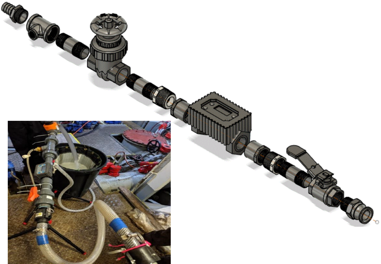
Figure 1 – Diagram and photo of the sample collection device
