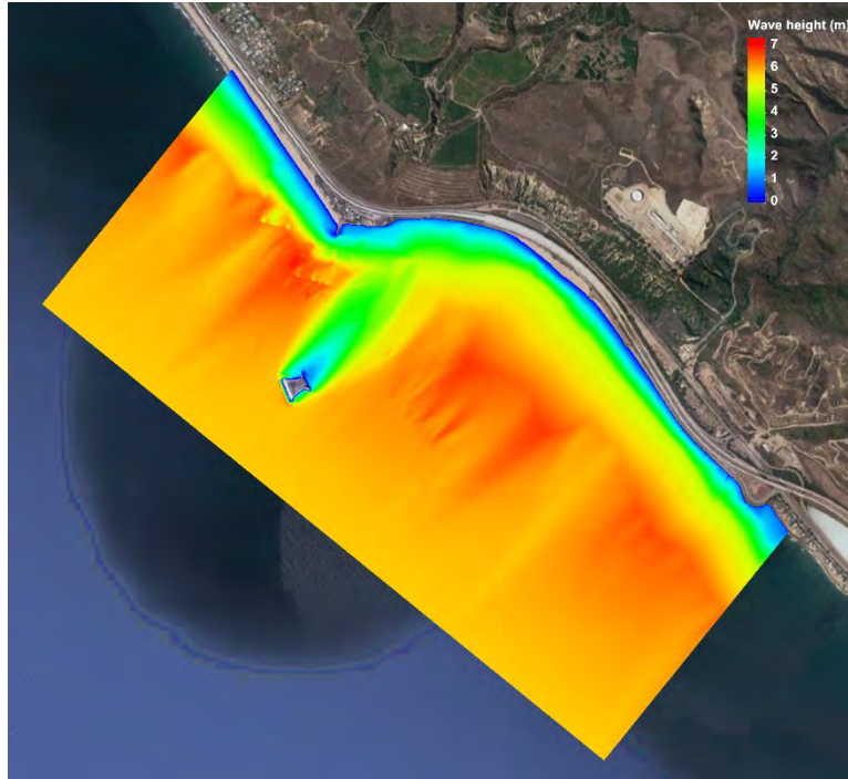
Figure 32. 50-Year Wave Height from SW, Existing Condition
