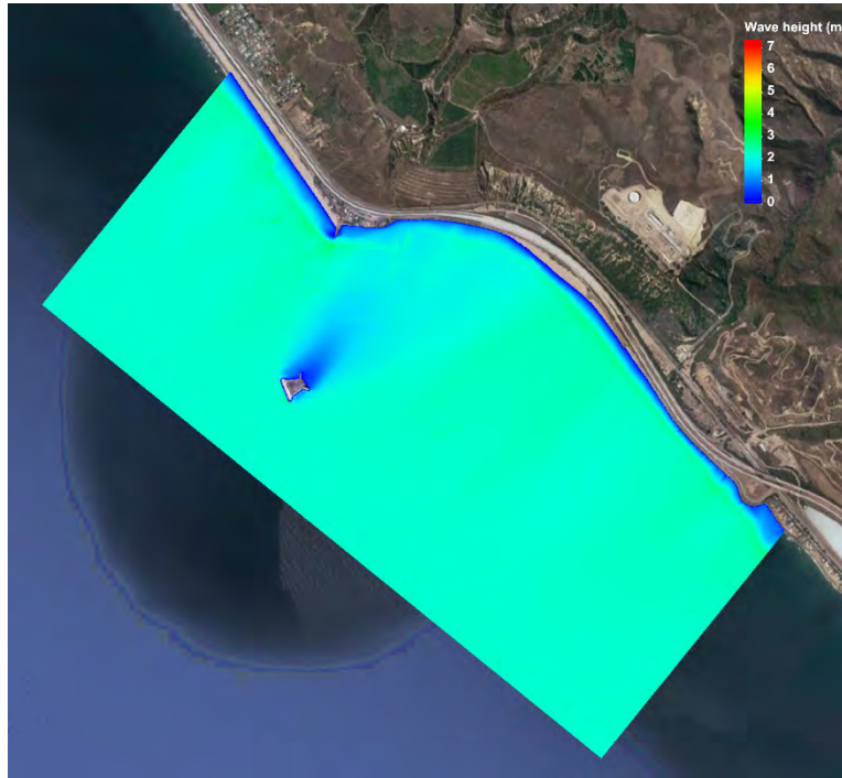
Figure 26. 1-Year Wave Height from SW, Existing Condition
