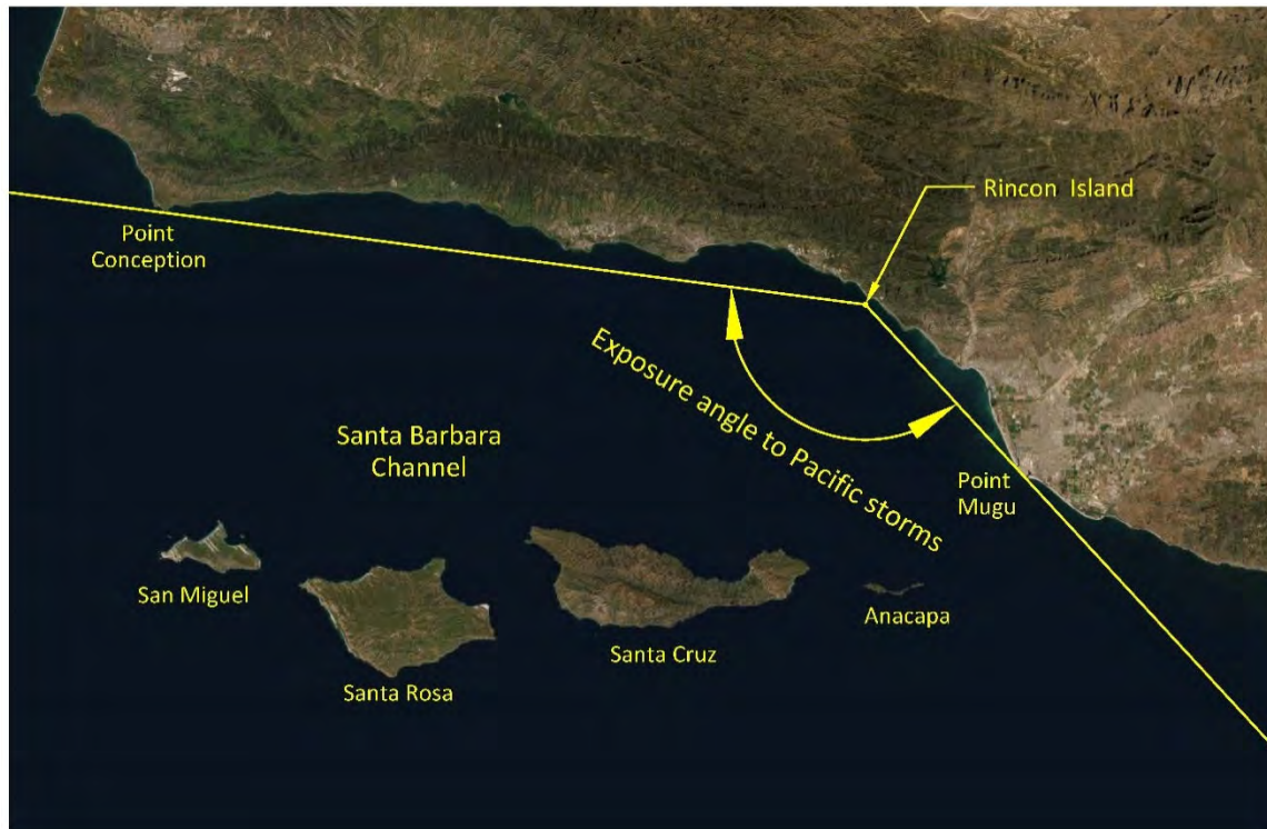
Figure 4. Rincon Island Exposure Angle to Pacific Storms
