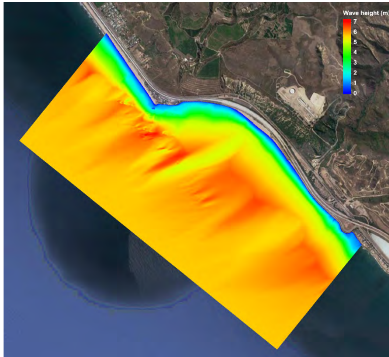
Figure 45. 50-Year Wave Height from WSW, Alternative 4
