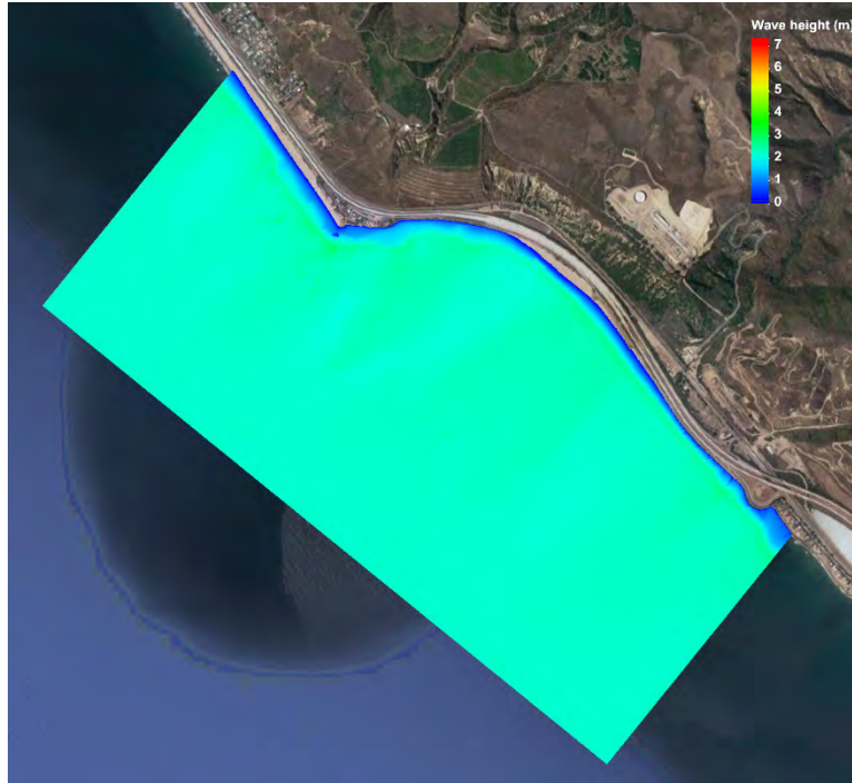
Figure 38. 1-Year Wave Height from SW, Alternative 4
