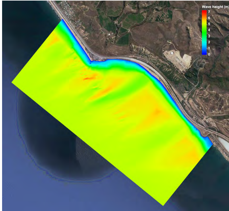
Figure 42. 10-Year Wave Height from WSW, Alternative 4
