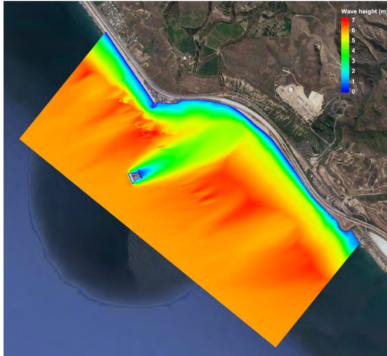
Figure 36. 100-Year Wave Height from WSW, Existing Condition
