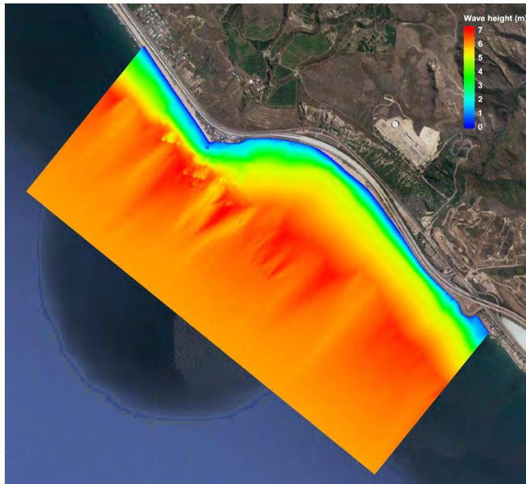
Figure 47. 100-Year Wave Height from SW, Alternative 4
