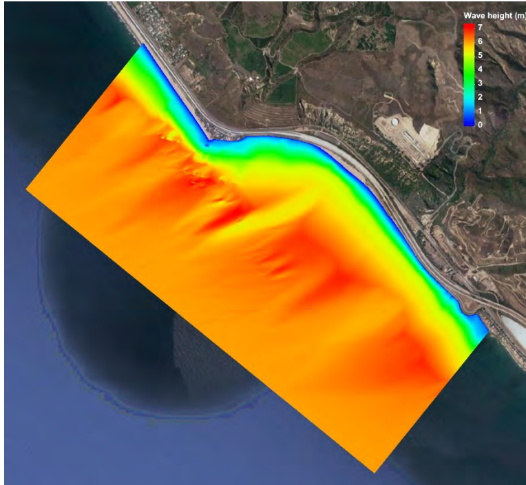
Figure 48. 100-Year Wave Height from WSW, Alternative 4
