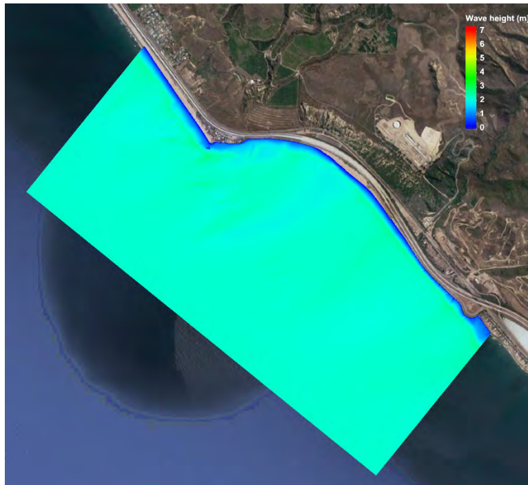
Figure 39. 1-Year Wave Height from WSW, Alternative 4
