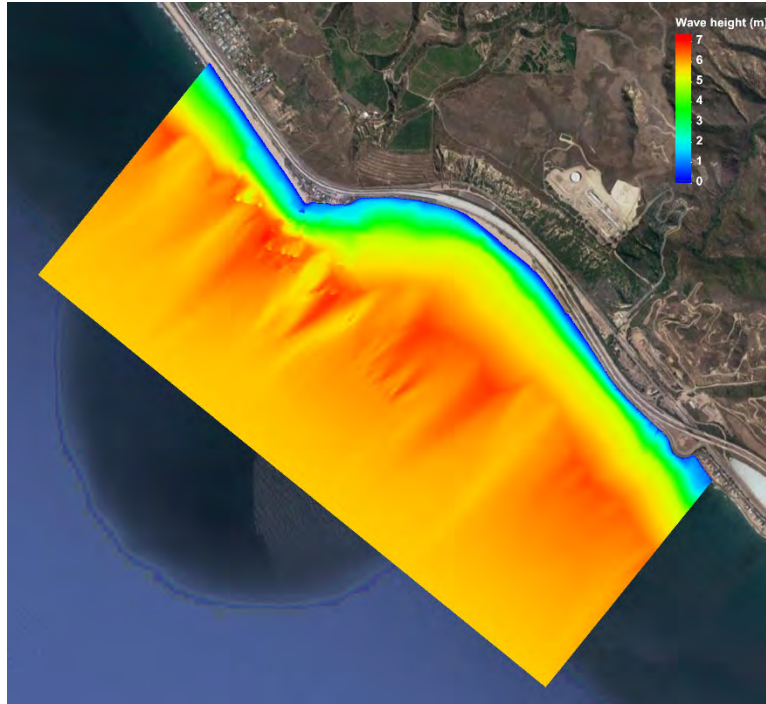
Figure 44. 50-Year Wave Height from SW, Alternative 4
