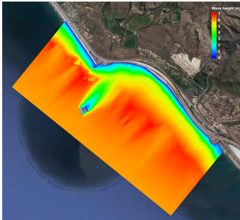
Figure 35. 100-Year Wave Height from SW, Existing Condition
