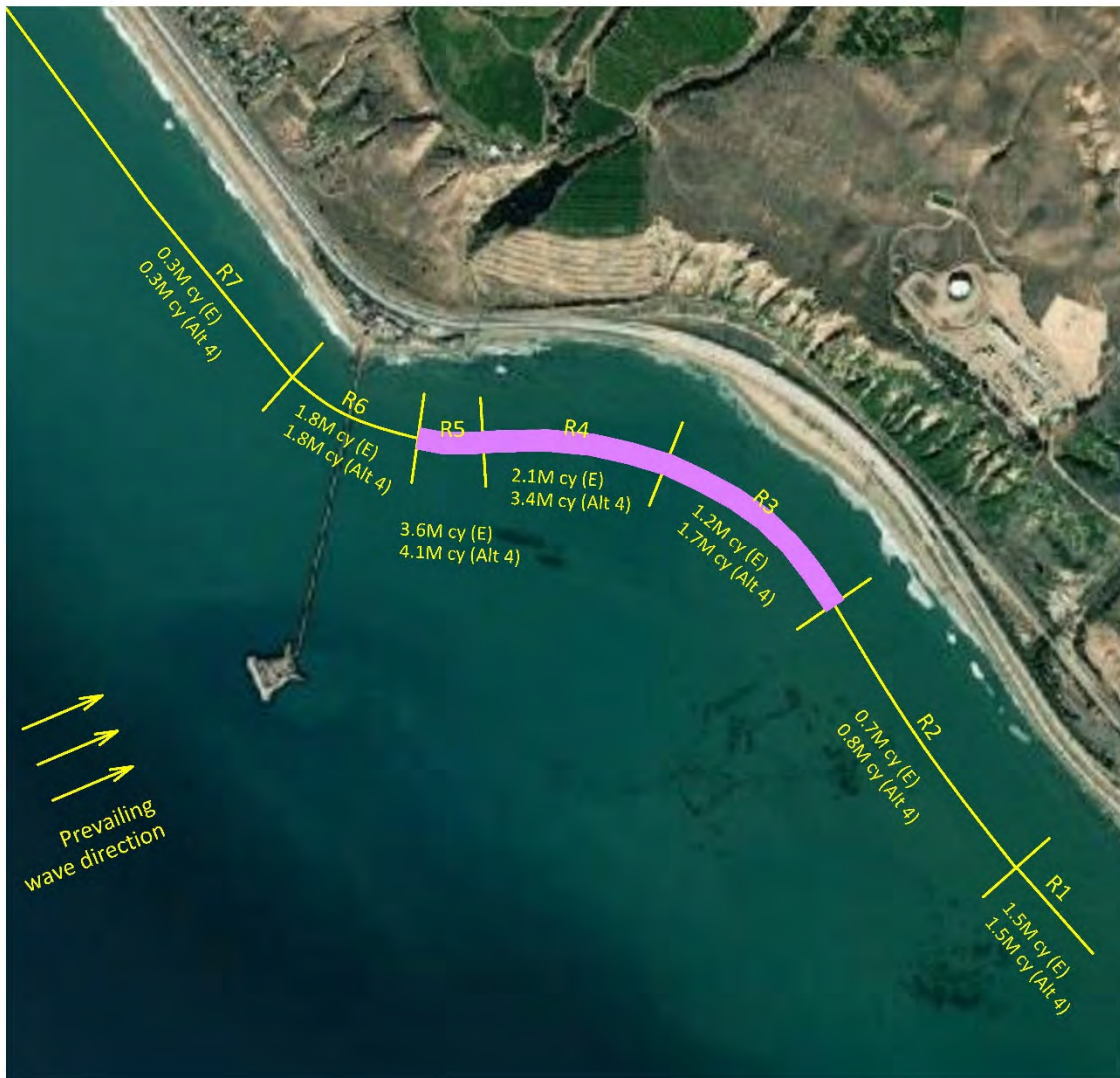
Figure 64. Alternative 4 Impact to Alongshore Sediment Transport Capacity
