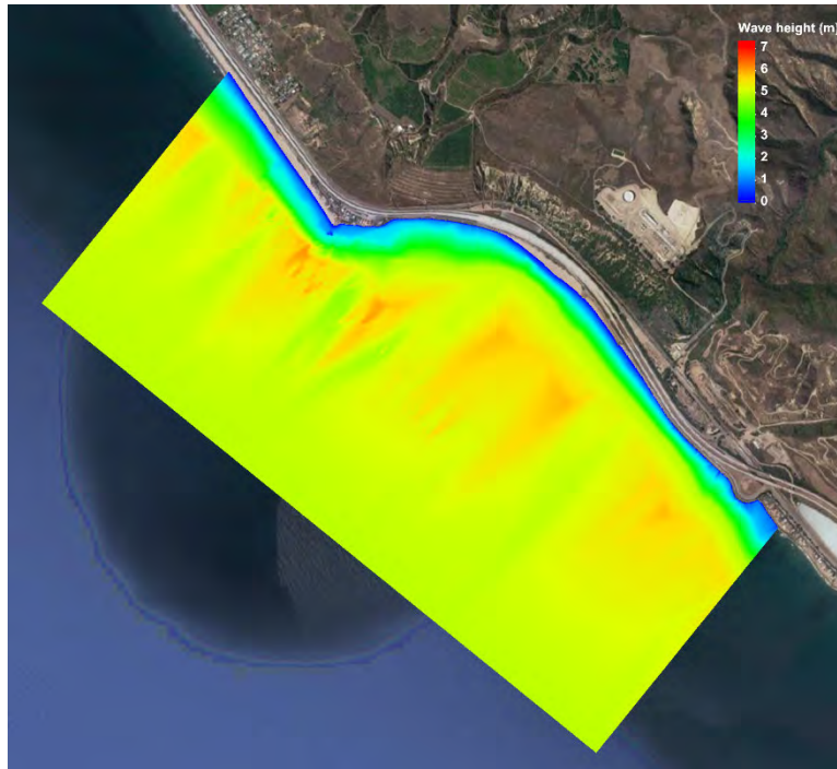
Figure 41. 10-Year Wave Height from SW, Alternative 4
