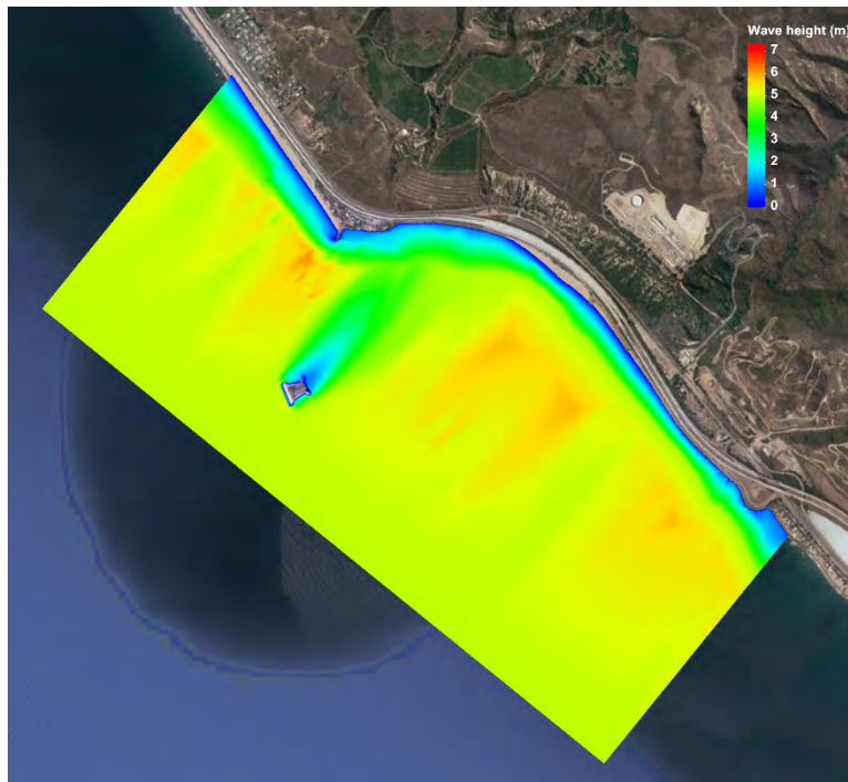
Figure 29. 10-Year Wave Height from SW, Existing Condition
