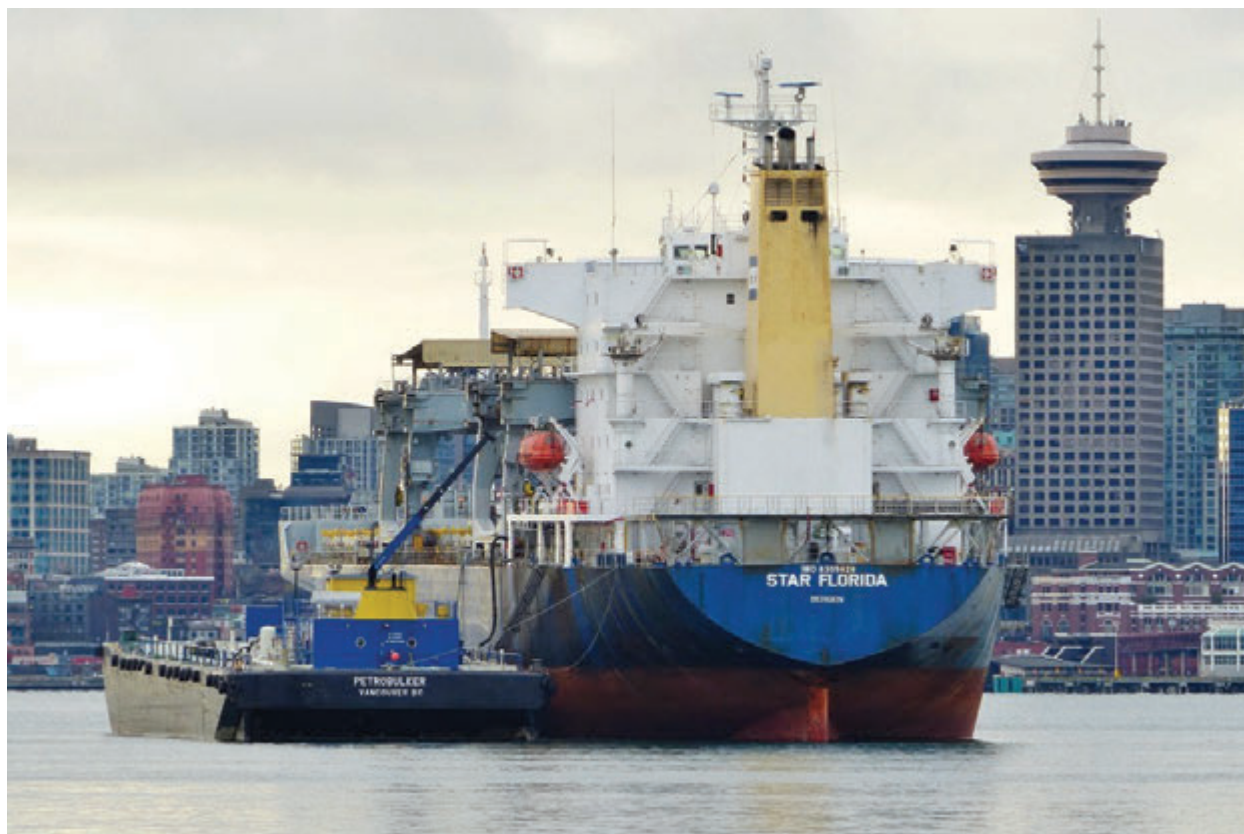
Figure 10 Open-hatch gantry ship, Star Florida engaged in bunkering operations in Vancouver Harbor, British Columbia.
