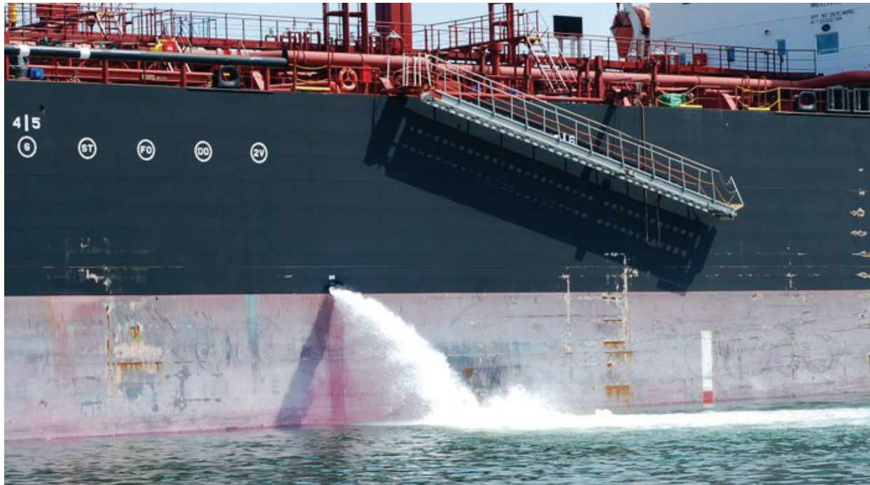
Figure 7 Overboard discharge from tankship at deep water line; the vessel is light and in ballast, so the overboard is above water line; if fully laden with cargo, the overboard would be at the water line
