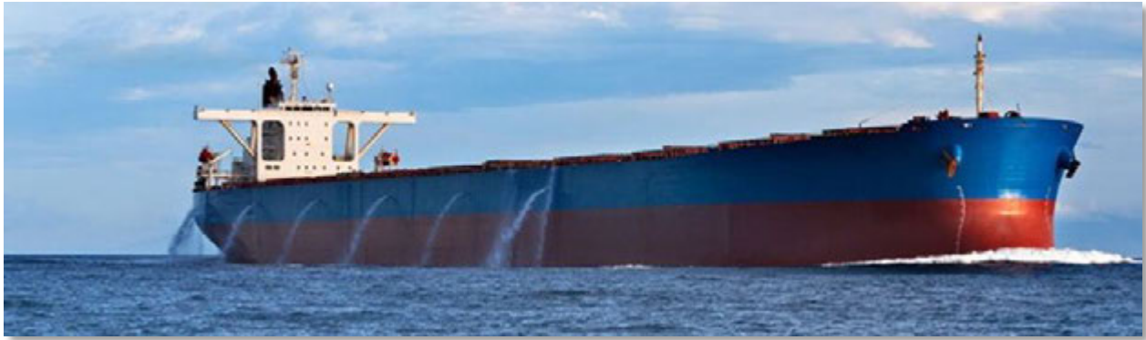
Figure 1 A dry bulk carrier discharging ballast while underway, in preparation for cargo operations (image from http://maritime-connector.com/ )
