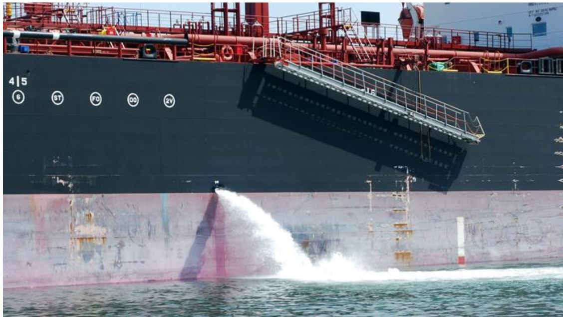
Figure 5 Overboard discharge from tankship located at deep water line; vessel is light and in ballast, so overboard is above water line; fully laden with cargo, and overboard would be at the water line
