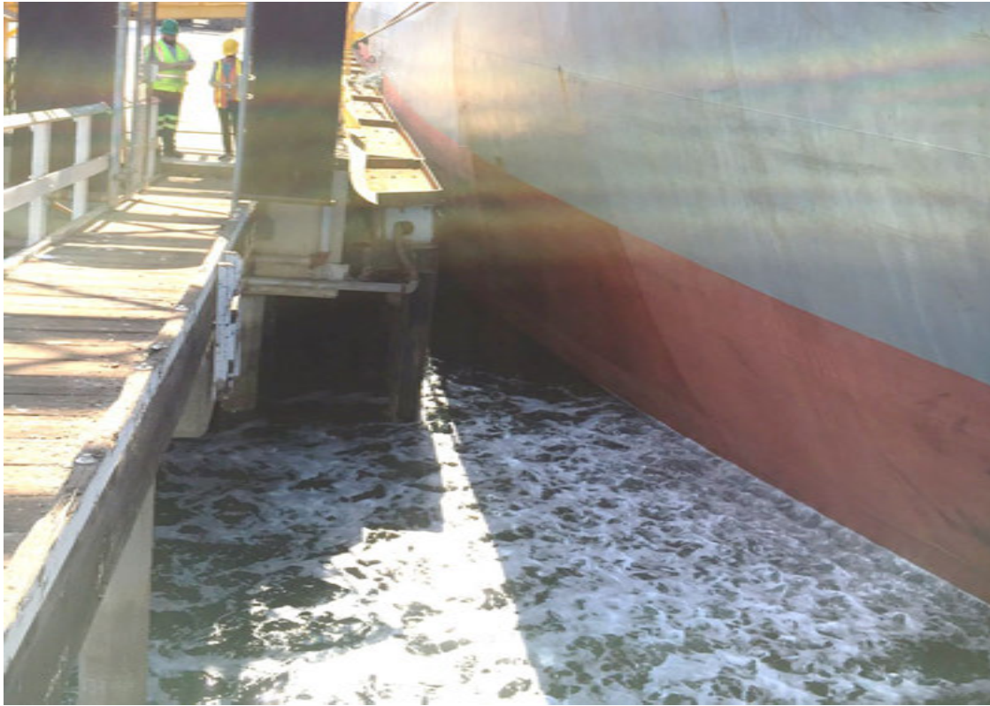
Figure 6 Bulk carrier discharging ballast through sea chest, well below water line
