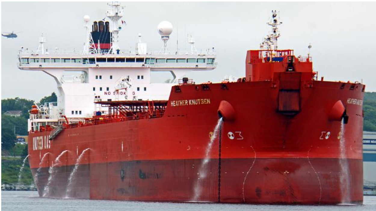
Figure 7 Very large crude oil carrier discharging ballast from multiple overboard pipes (image, wikimedia commons accessed 19 September 2017)
