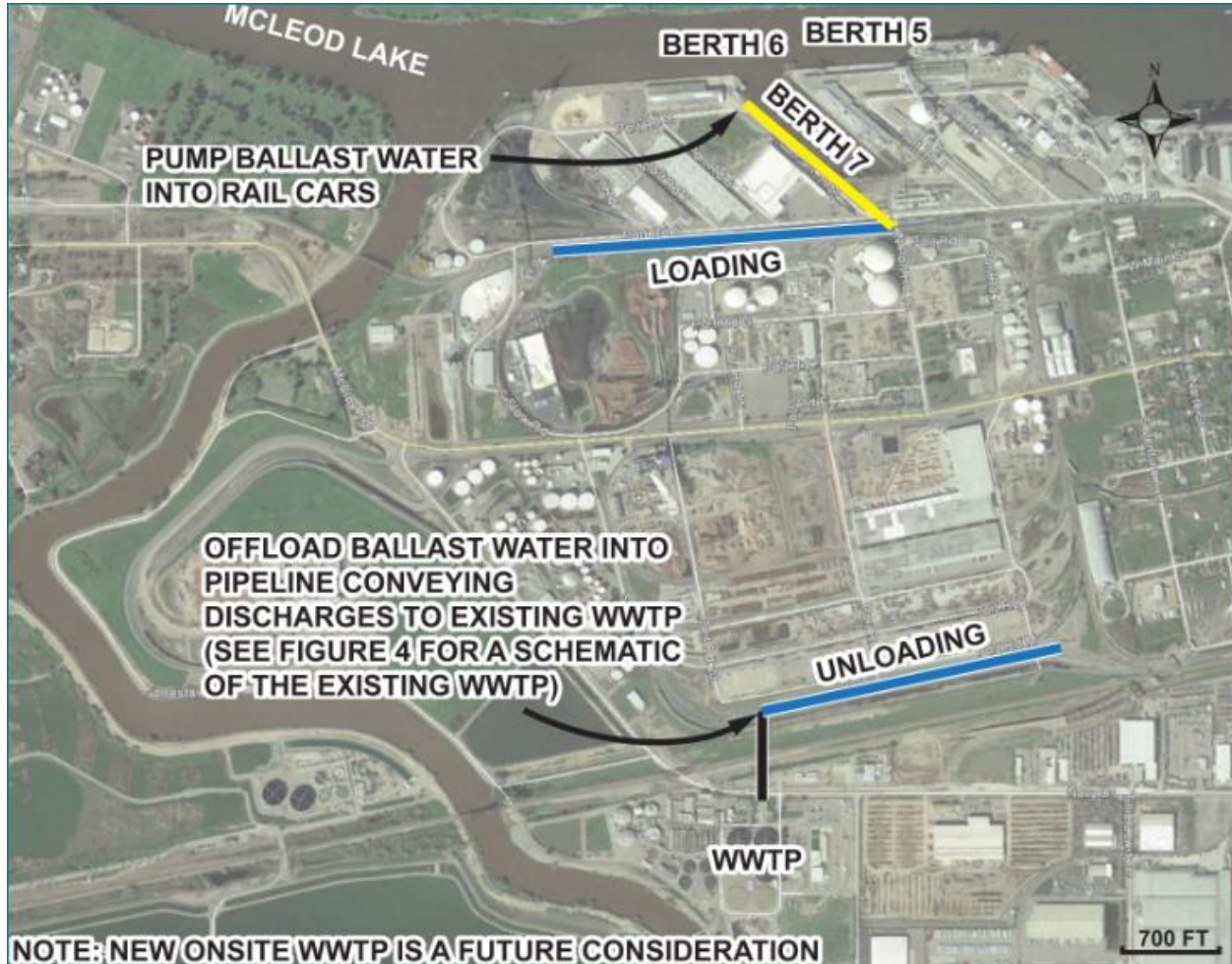
Figure 7 Port of Stockton/east complex rail car conveyance conceptual approach
