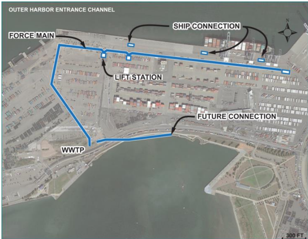
Figure 12 Port of Oakland TraPac Terminal conceptual conveyance approach
