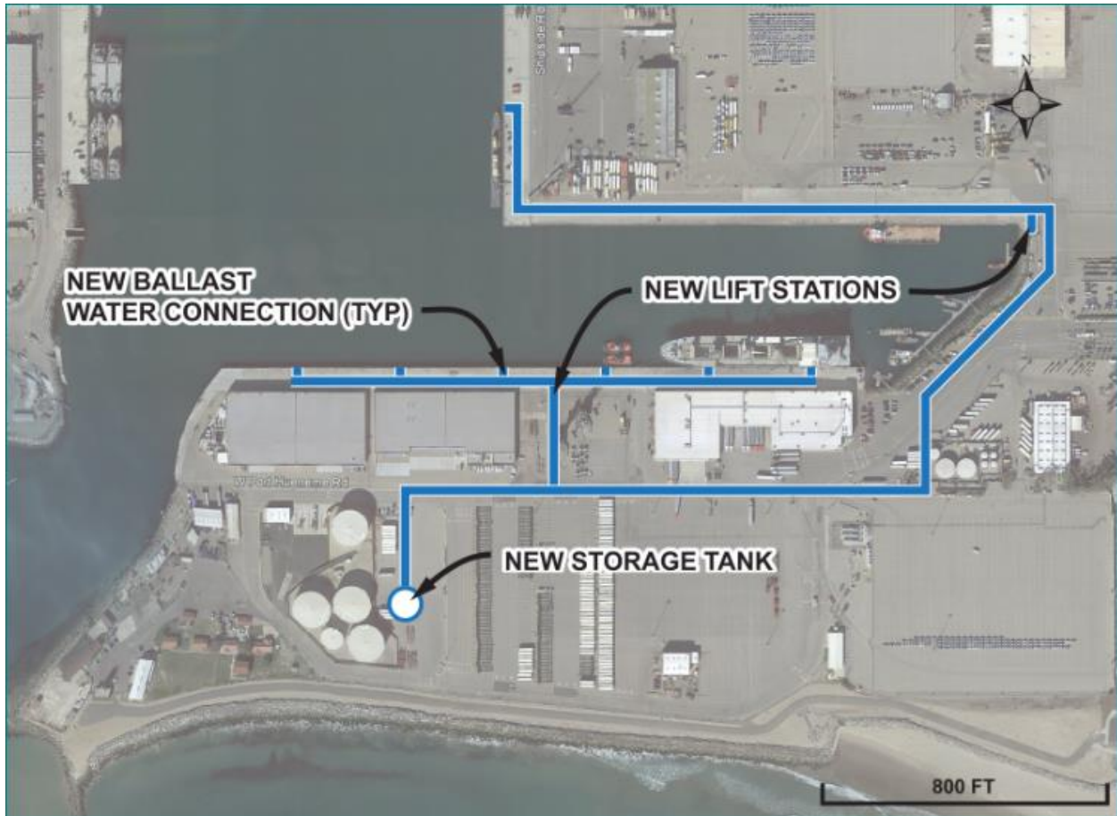
Figure 16 Port of Hueneme Terminal conceptual conveyance approach
