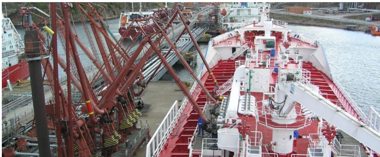
Figure 1 Brofjorden marine terminal. Loading arms are similar in size to that needed for SA Recycling ballast water handling operations, but smaller than required for Stockton or El Segundo case studies. (Marcus Bengtsson, wikicommons)
