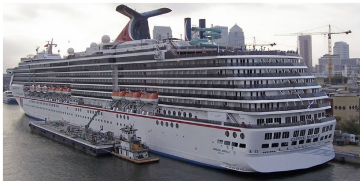
Figure 30 Aerial view of the 3,054 passenger and crew Carnival Miracle , taking fuel oil bunkers by barge (image, FleetMon.com)
