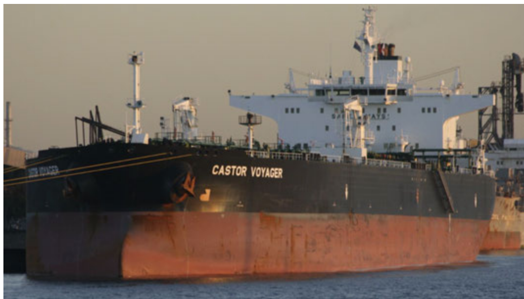
Figure 26 Tankship Castor Voyager at 105,000 deadweight, estimated ballasting at 3,400 m 3 /hr
