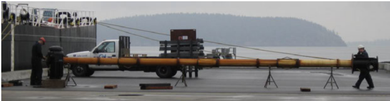
Figure 16 Typical deepwell pump being serviced dockside
