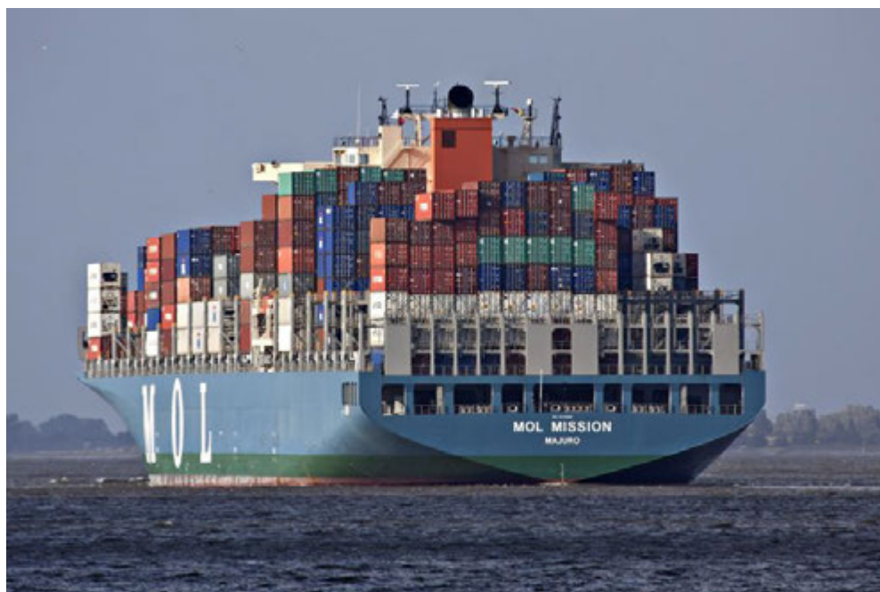
Figure 19 6,724-TEU containership MOL Mission , which calls at Port of Oakland (image, Klaus Kehrls)
