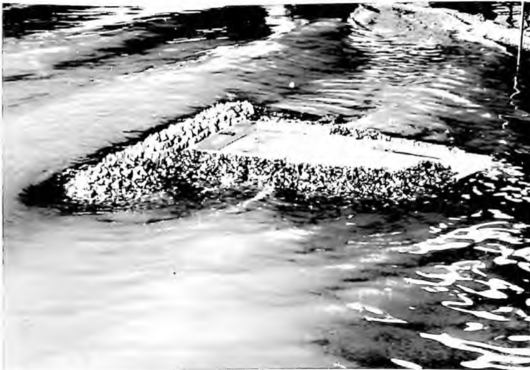
Fig. 9. Three Dimensional Wave Action Test.
