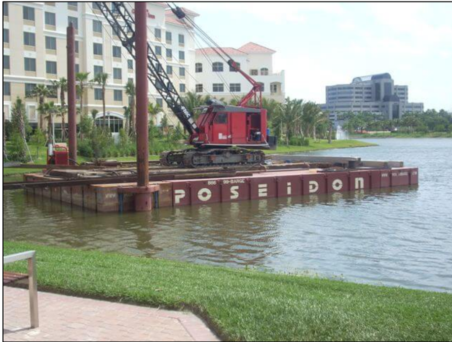
Figure 2-8. Example Use of a Sectional Barge with Crane
