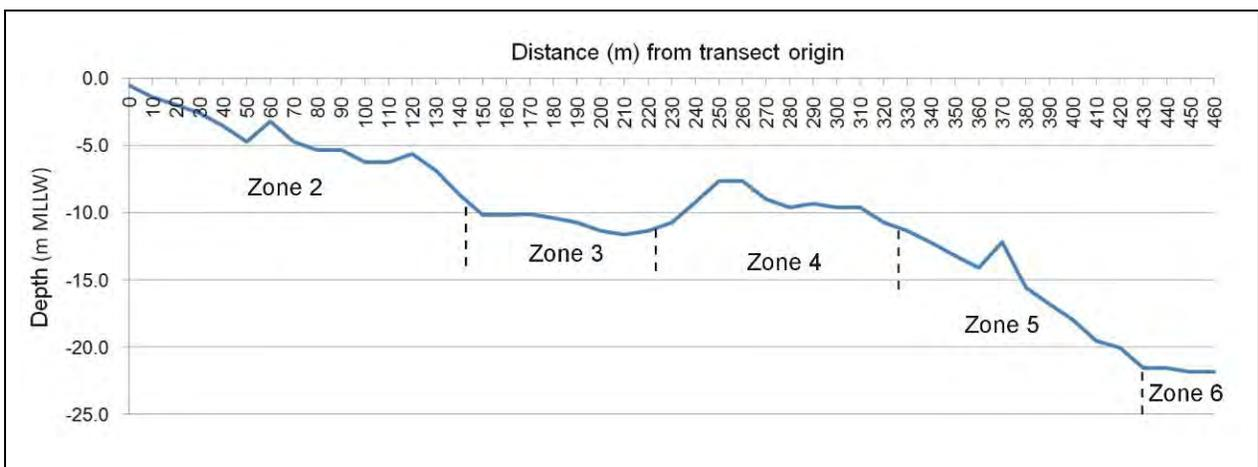
**Figure 3.** Depth profile of the subtidal survey transect showing locations of general habitat zones described in Figure 2. Vertical exaggeration of the depth scale is approximately 6:1.
