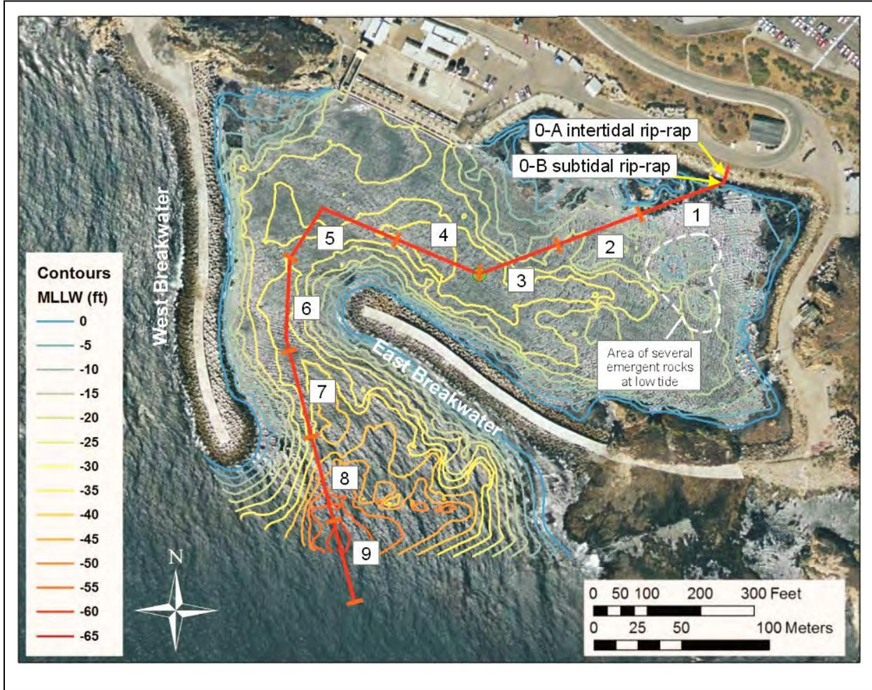
**Figure 1.** Proposed OBS cable corridor route (red line) and transect segments surveyed through the DCP intake cove on May 17–20, 2011. Depth contours are from multi-beam hydroacoustic surveys conducted in 2005.
