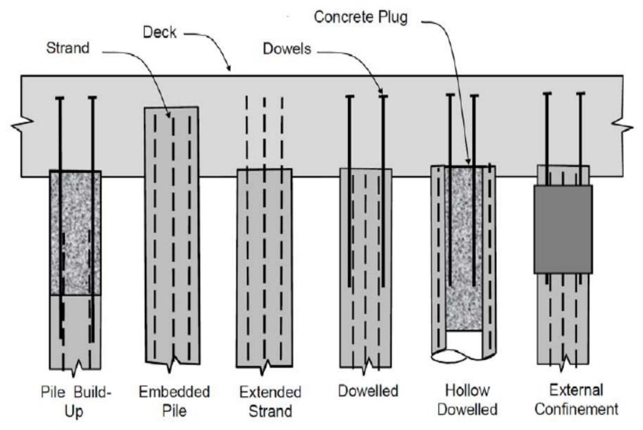
Figure C7.5 Examples of prestressed concrete pile connections
